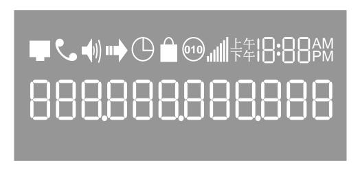
The LCD is equipped with a backlight. When the phone is configured properly and in the normal idle state, the backlight is off. Whenever an event occurs, the backlight turns on automatically and brings the user's attention.
